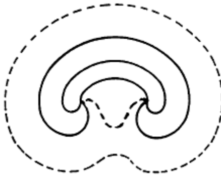
Figure 4.19 The Frank-Read source: a straight portion of edge dislocation is anchored at its ends by screw dislocations of opposite sign. Under stress the edge dislocation successively bows out as shown; eventually it meets up with itself and generates a closed loop, but at the same time the original dislocation is reformed (broken line) which allows a continued production of loops.
