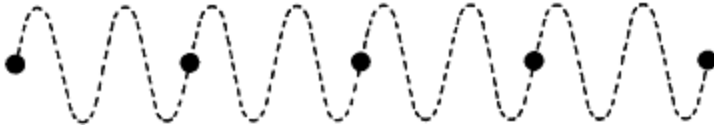
Figure 5.7 The wave profile for \omega=0 , k=4\pi/a . The wave form coincides with the positions of the masses only at certain nodes.
