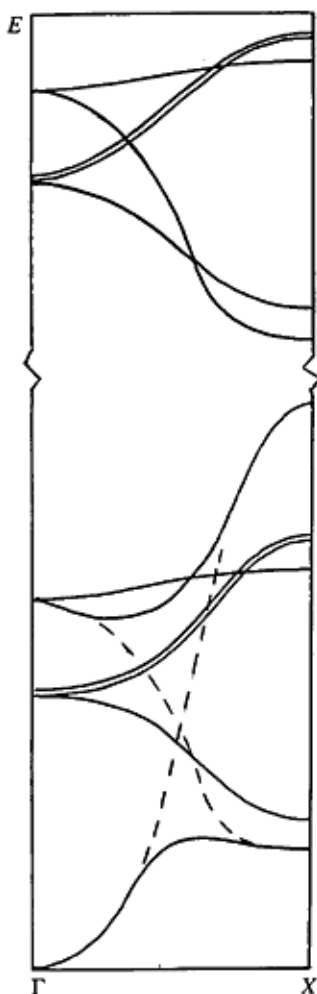
Figure 7.22 The five d sub-bands of a transition metal atom arise on account of interatomic overlap of orbitals centred on neighbouring atoms; each of the five orbitals produces a narrow sub-band with its own characteristic dispersion (upper part of figure). It is not obvious why the different bands disperse as they do, and we take the above shapes for granted. The d electrons, however, overlap the valence electron states in both space and energy, and this leads to a hybridization or mixing of the states—this is the s-d resonance described in the text. The lower part of the figure shows the result of this mixing. Only one of the d sub-bands is strongly affected—a consequence of the symmetry dependence of the hybridization. The underlying unhybridized d sub-band and sp conduction band are shown as broken lines. This diagram shows the behaviour only in the \Gamma X direction in the fcc structure; Fig. 7.25 shows the complete band diagram for this crystal structure. (After Mott 1964.)
