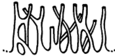
Figure 10.18 An impression of the structure of the porous Si layer on an electrolytically etched single crystal Si wafer. The individual filaments have diameter \sim \text{nm} and length \sim \mu\text{m} . (After Canham 1992.)
